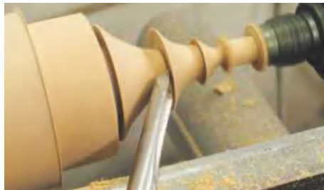
▲ Pic.5 Keep the flute at 2 o'clock as the gouge runs down the curve. The flute will need to go over to 3 o'clock as you near the larger diameter
